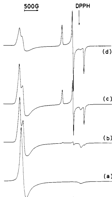
Figure 1. EPR spectra at 25 K of Fe(TPP)Cl in toluene-methanol (5:2 v/v) in the absence or presence of the MeO - anion: [Fe(TPP)Cl] 0 = 1.4 × 10 -3 M, [MeO - ] 0 /[Fe(TPP)Cl] 0 = 0 (a), 2 (b), 10 (c), and ~50 (d). The spectra indicate three complex species in the solutions. They are assigned to Fe(TPP)Cl (high spin; g_x = g_y = 6.03 , g_z = 2.00 ), Fe(TPP)(OMe) (high spin; g_x = 5.55 , g_y = 6.40 , g_z = 1.99 ), and Fe(TPP)(OMe) 2 - (low spin; g_x = 1.914 , g_y = 2.165 , g_z = 2.494 ) with the spin state and g values in parentheses.
